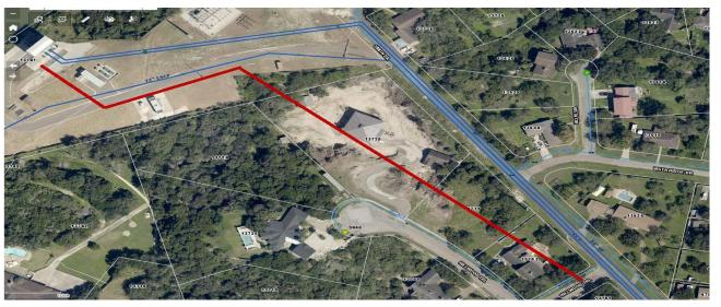
Project Phase 2 - The red line shows the proposed alignment for the new 54" water transmission main from the Nueces River Pump Station to the connection point on Smith Drive. Staff recommends purchasing properties to allow the City to construct the new line by open trench and negate 600 - 750 feet of tunneling and save more than \$5 million in construction costs. This will also protect the City's water infrastructure.
