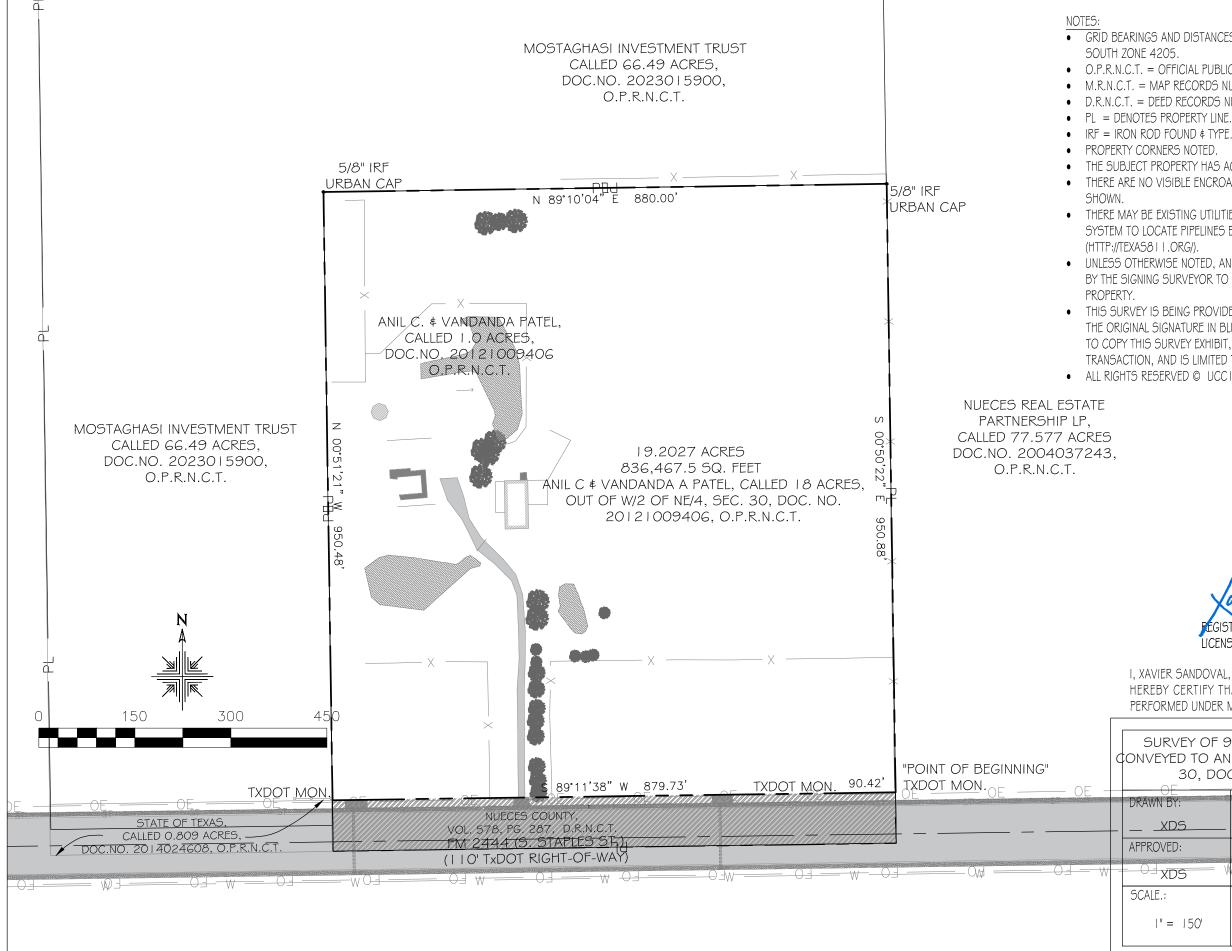
• GRID BEARINGS AND DISTANCES ARE REFERENCED TO THE TEXAS COORDINATE SYSTEM, NAD83.
