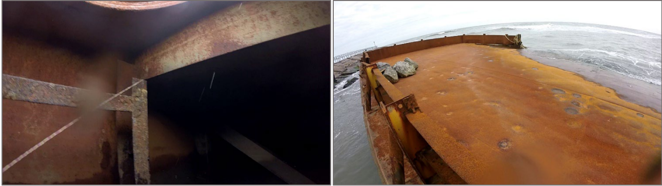
Figure 5 Barge Deck and Internal Structure Appear in Good Condition
