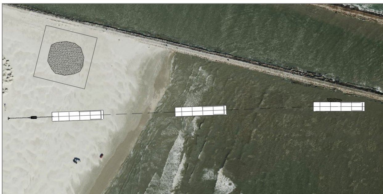
Figure 11 Beginning, middle, and end of pulling operation
