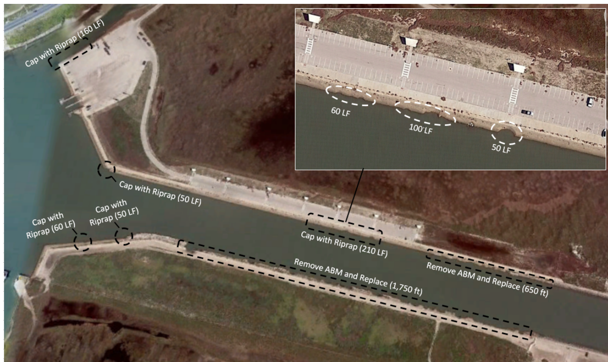
Figure 9 – ABM Damage Areas and Repair Classifications in Reach 3.
