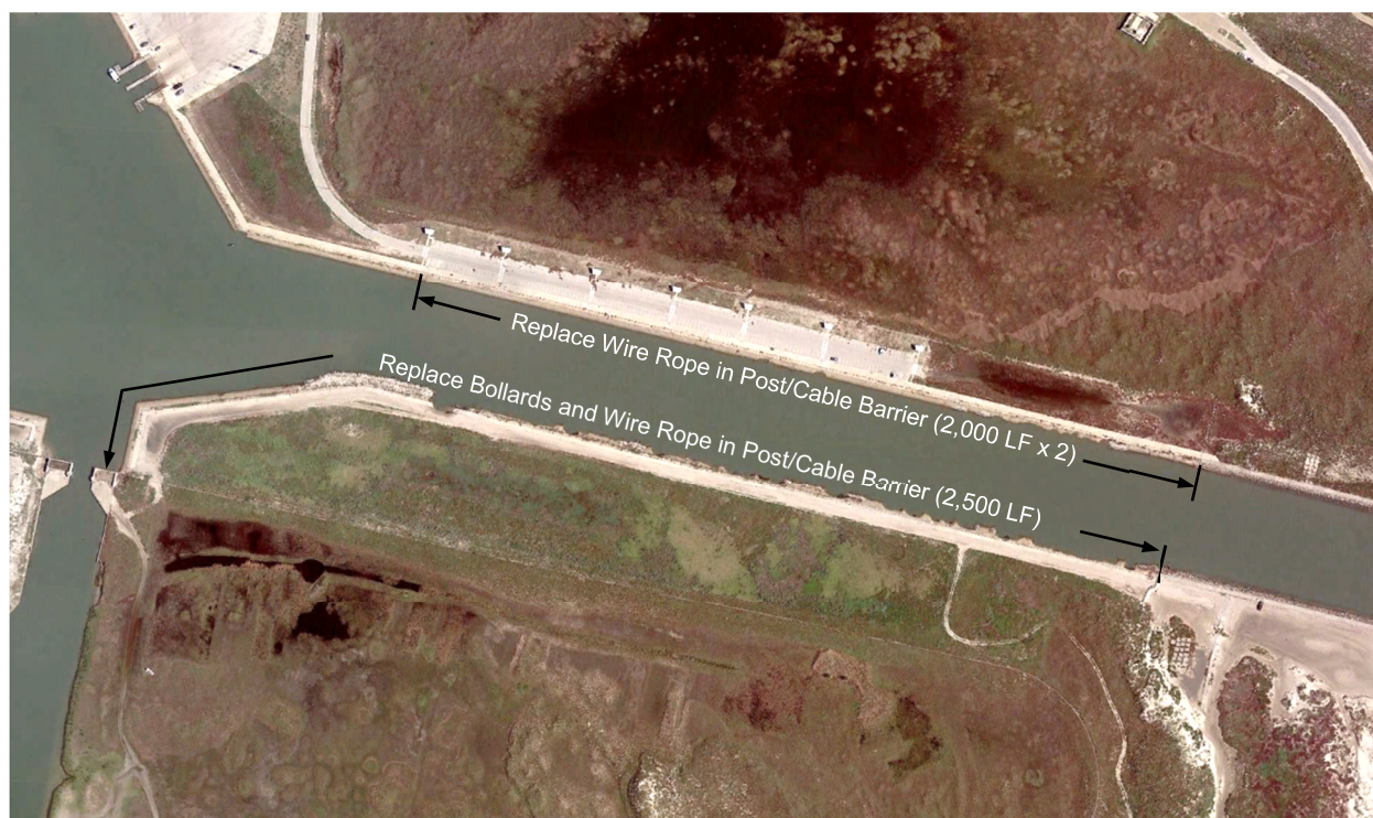
Figure 14 – Harvey Repair: Post/Cable Barriers.
