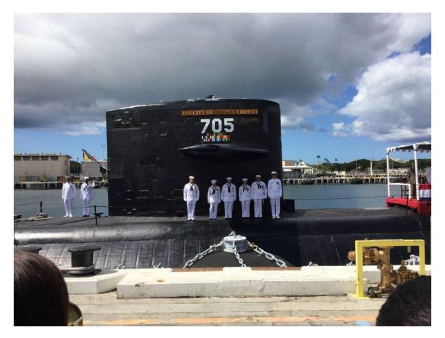
Physical Description SSN705 Length: 26 ft 3 In Height: 17 ft Width: 5ft (excluding fairwater planes) 30 ft (including fairwater planes) Weight: approx. 120,000 lbs (60 tons) with fairwater planes installed
