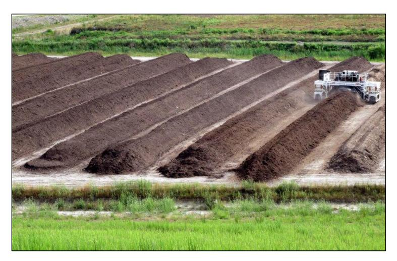
The proposed compost facility will process wood chips mixed with wastewater sludge in an Aerobic, open windrow format
