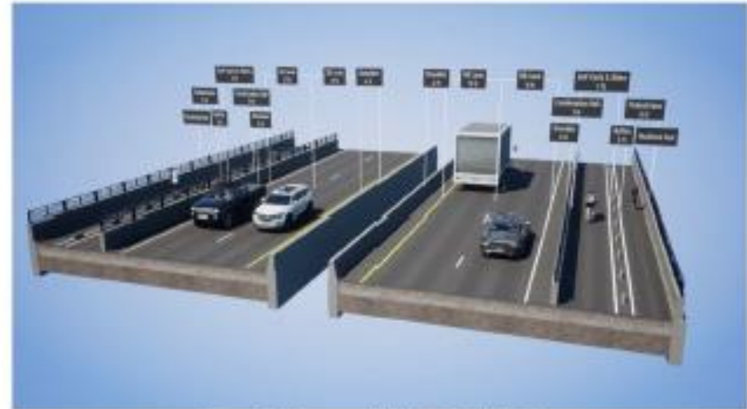
Figure 3: Proposed Bridge Typical Section
