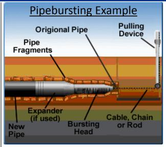
A bursting head is pulled through the existing pipe effectively breaking the old pipe into pieces and expanding the cavity allowing the new pipe to be simultaneously pulled into place behind the bursting head.
