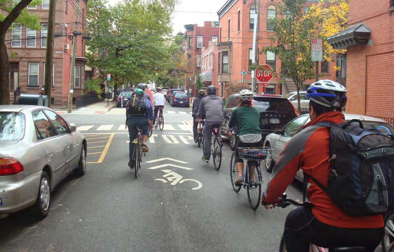
▲ BIKE BOULEVARD WITH SHARROW SYMBOL. HOBOKEN, NJ BICYCLE BOULEVARD ▼ BIKE BOULEVARD WITH DIVERTER. PORTLAND, OR
