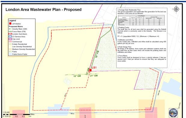
This plan is consistent with the Wastewater Master Plan Trunk Line System for the London Service Area.
