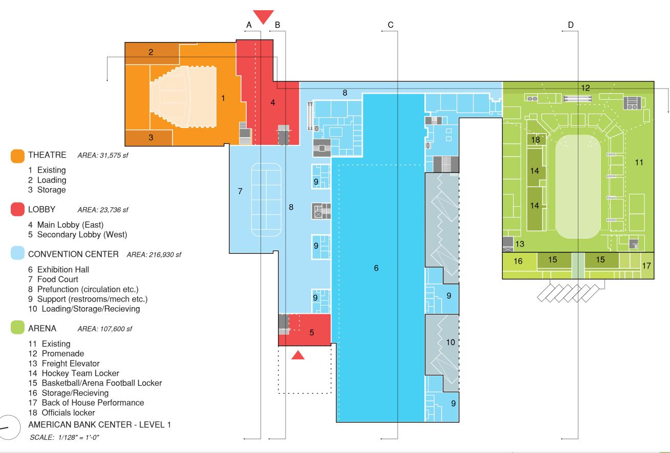
Level 1 Plan showing revisions to the theater, entry lobby sequence, and pre-function and food court zones of the convention center. The exhibit halls are also expanded to the west and include new dock and support/loading space. The arena includes a proposed lobby expansion to accommodate circulation from the south hotel site as well as renovations to existing locker rooms, a new freight elevator and expanded support to the west to accommodate additional facilities.
