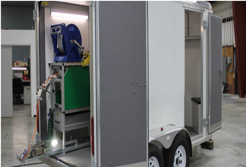
Rausch C90 HD Mobile Pro Camera Cube Trailer CCW Wastewater Qty: 1
