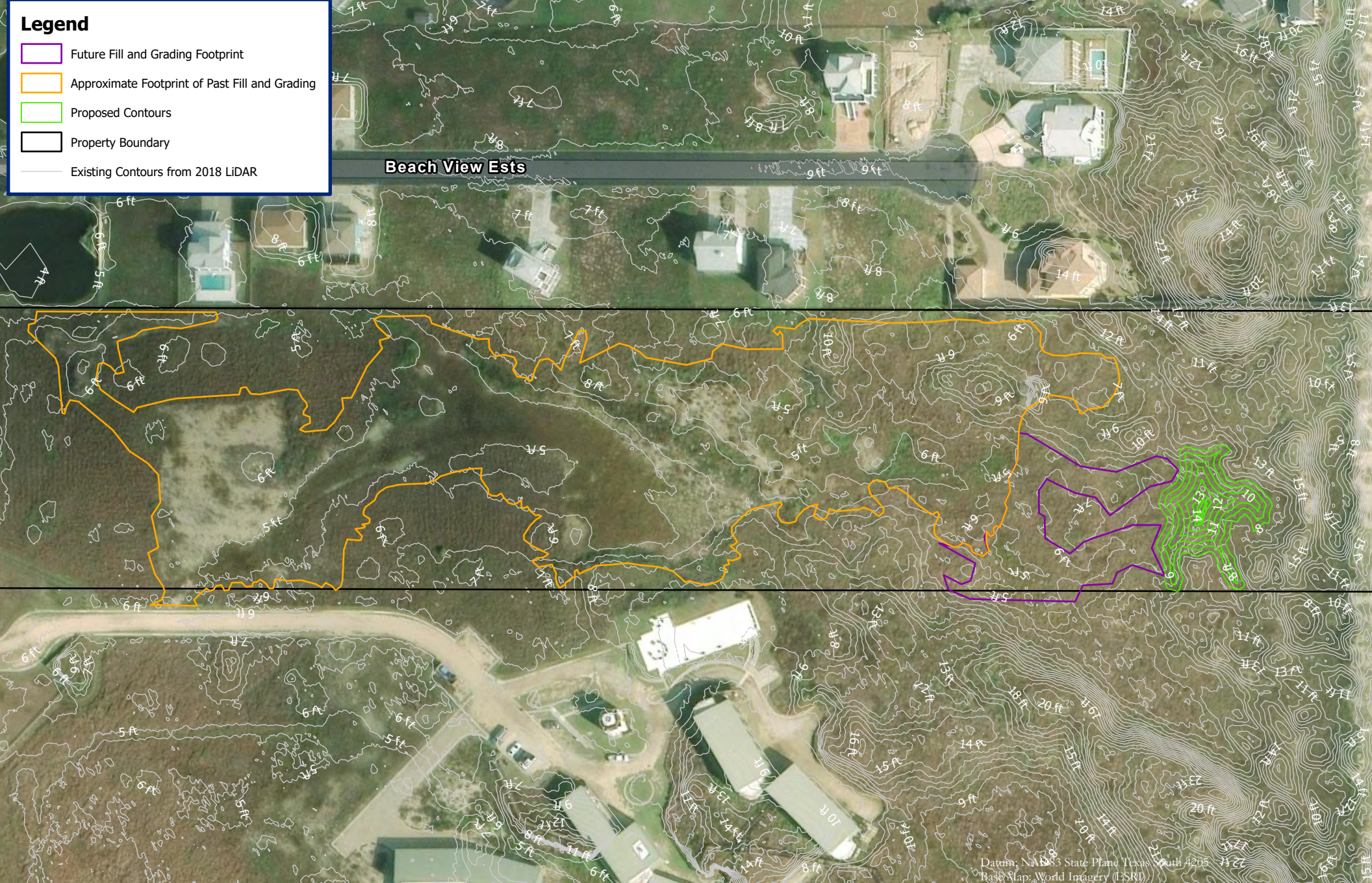
Figure 2 - Grading and Layout Plan
