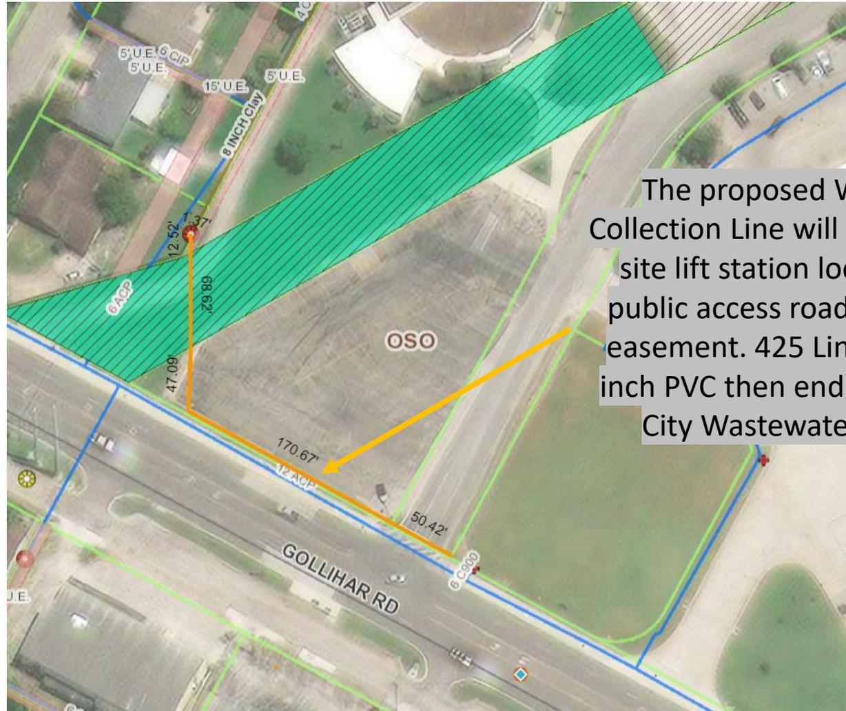
The proposed Wastewater Collection Line will begin at an on-site lift station location near a public access road/public utility easement. 425 Linear Feet of 2-inch PVC then end at an existing City Wastewater manhole.
