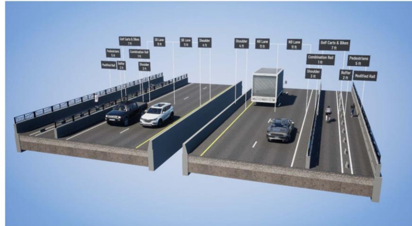
Figure 3: Proposed Bridge Typical Section
