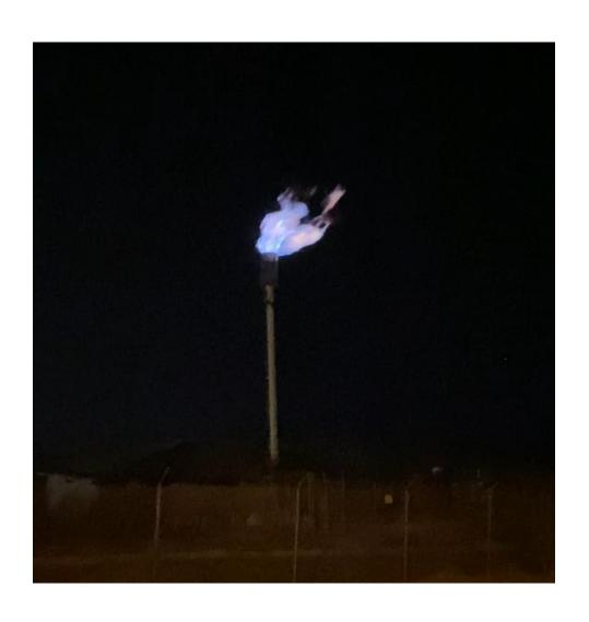
Landfills are some of the largest emitters of green house gases and are highly regulated by the EPA. To meet EPA and TCEQ rules and regulations the landfill gas is burned in flares at both Cefe and J.C. Elliot.
