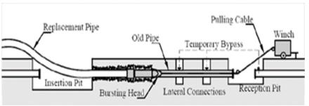
Pipe bursting is a well-established trenchless method that is widely used for the replacement of deteriorated pipes with a new pipe of the same or larger diameter. Pipe bursting is typically cost-effective if the existing pipe is deep, below the ground water table (GWT), and the existing pipe is undersized. Pipe bursting is also an effective alternative to reduce disturbance to streets, business and residents verses open cut technique.
