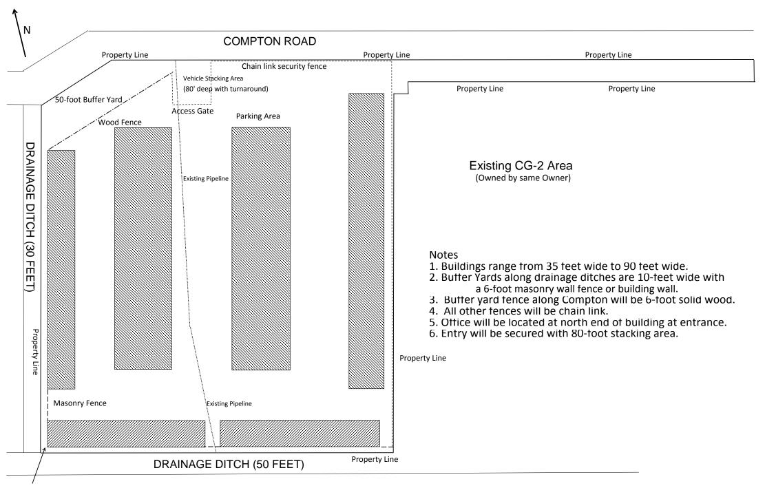
10-foot buffer yard between masonry wall and property line.
