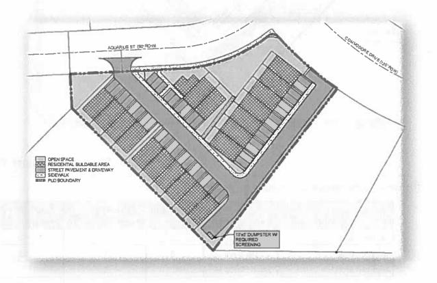
The Vehicular and Pedestrian Access for the development is indicated below. The entrance into the development will provide a 24 foot clear entrance/exit for emergency vehicles. The private drive within the development will be a minimum of 22' wide from edge of pavement throughout with fire land striping and signage installed. The development will provide a sidewalk and additional sidewalks may be provided to promote walkability and access to amenities that are not indicated.
