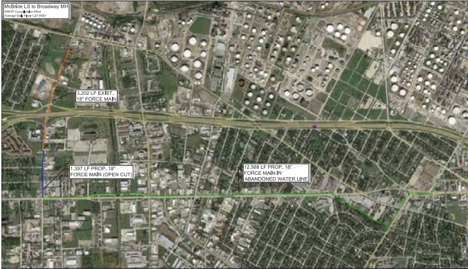
Figure 2-5 Potential Force Main Routing for Flow Diversion from Arcadia Lift Station to Broadway WWTP
