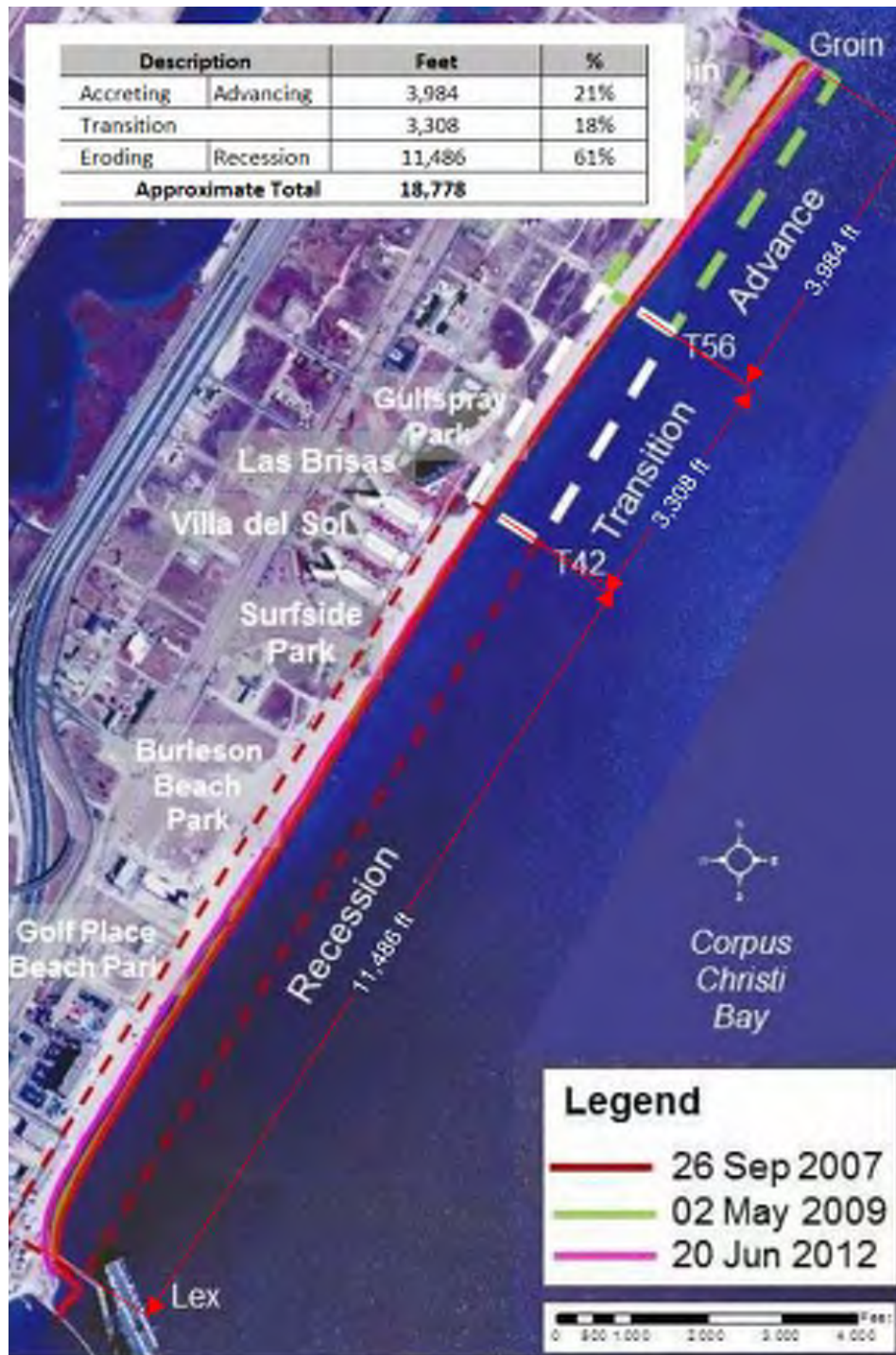
Figure 11-6. North Beach Erosion Rates 2007 to 2012 15
