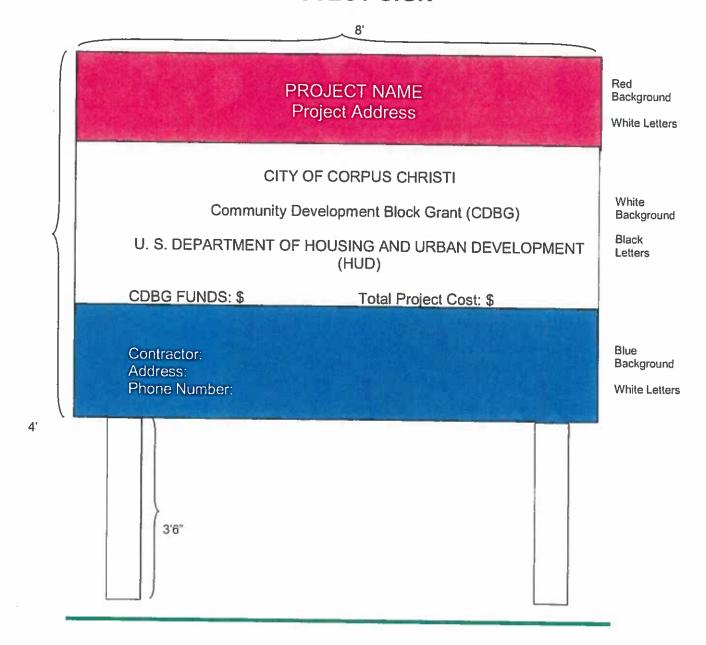
Contractor to locate sign where it is most visible to the public and as approved by City Sign is made from a 4 feet x 8 feet sheet of ¾" plywood.
