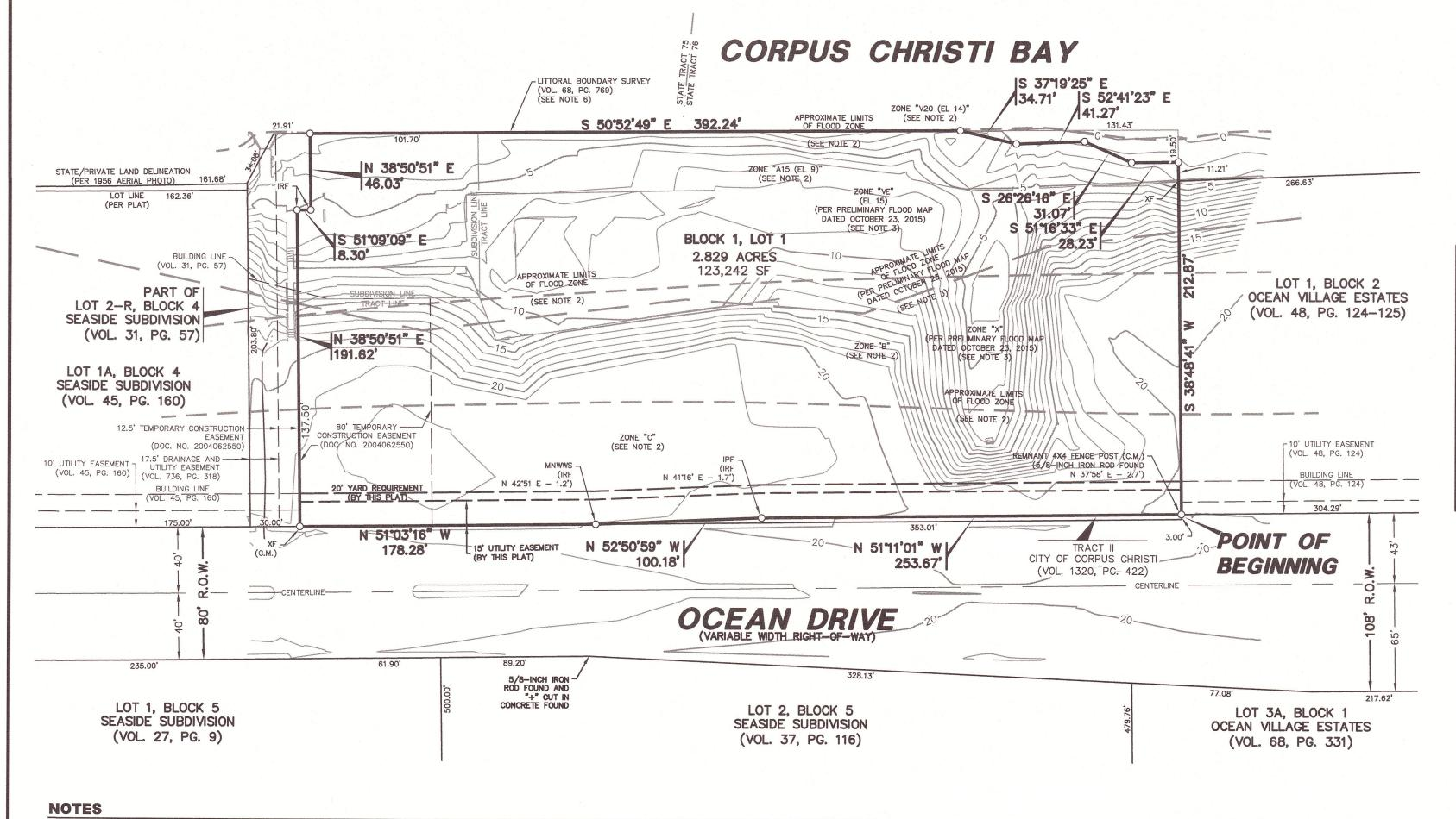
1. Bearing system for this survey is based on the State Plane Coordinate System, North American Datum of 1983 (2011), Texas South Zone 4205.
