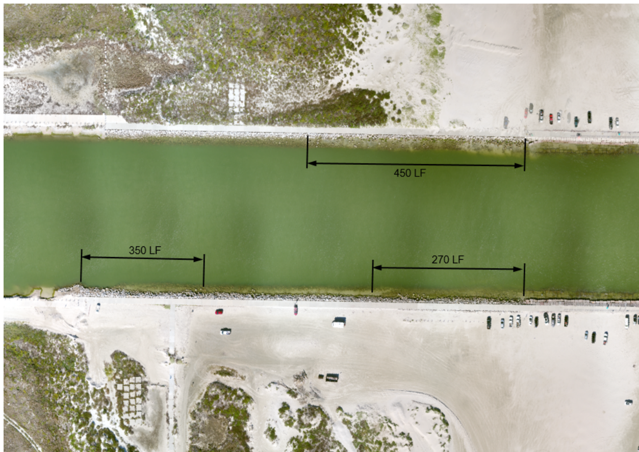
Figure 15 – Landside Jetty Damage Areas in Reach 2.
