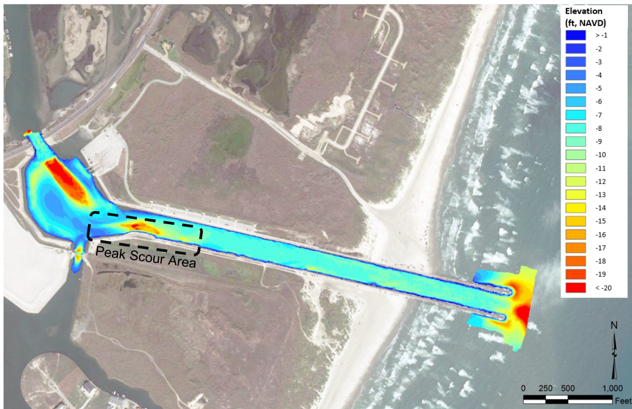
Figure 5 – Survey Showing Bottom Elevations in Packery Channel after Hurricane Harvey (Survey performed by Naismith Marine Services, Inc. during September 2017).
