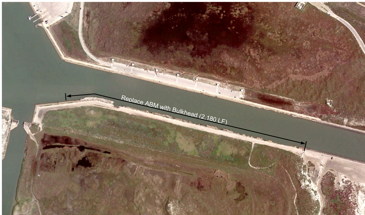
Figure 21 – Hazard Mitigation, Reach 3, Option 3 (Replace ABM with Bulkhead).
