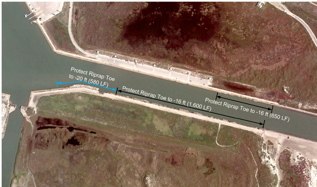
Figure 19 – Hazard Mitigation, Reach 3, Option 2 (Replace ABM with Riprap Revetment).
