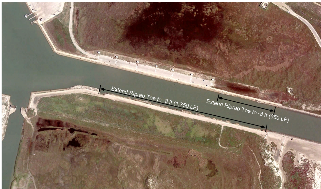
Figure 17 – Hazard Mitigation, Reach 3, Option 1 (Replace ABM with Riprap Revetment).
