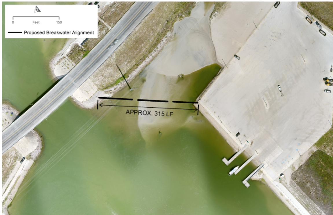
Figure 23 – Approximate alignment of riprap breakwater concept in Reach 4 (breakwater gap locations and dimensions to be determined).
