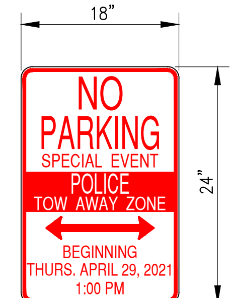
TYP. NO PARKING SIGN MOUNT ON REFLECTORIZED DRUM
