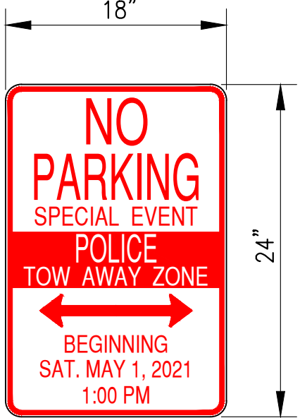
TYP. NO PARKING SIGN MOUNT ON REFLECTORIZED DRUM AS LOCATED
