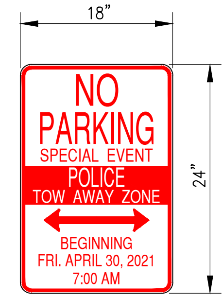
TYP. NO PARKING SIGN MOUNT ON REFLECTORIZED DRUM AS LOCATED
